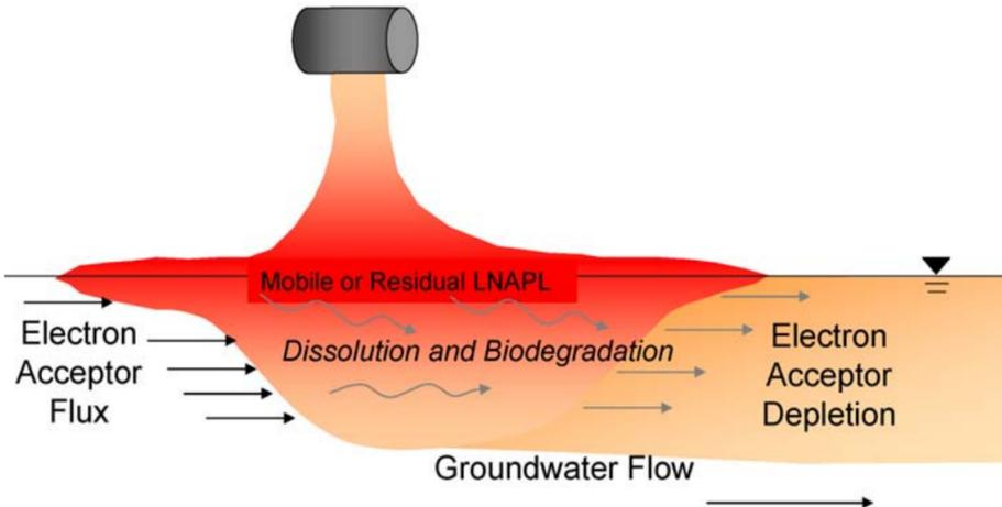
Figure 1: LNAPL mass depletion processes in submerged source zone (from ITRC, 2009).
