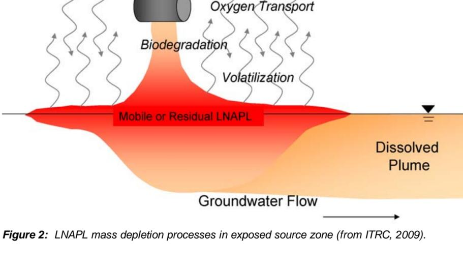
Figure 2: LNAPL mass depletion processes in exposed source zone (from ITRC, 2009).
